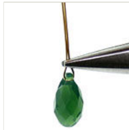
Step 5 Hold the two wires with your chain nose pliers just above the tip of the briolette.
