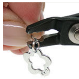
Step 5 Turn the bead a quarter turn and place the crimp bead in the front notch.
