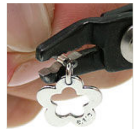
Step 3 Make sure that the wires are lying parallel to each other. Place the crimp bead into the back notch.
