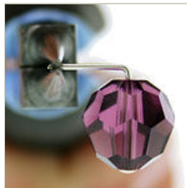
Step 4 Grasp the end of the wire with round nose pliers so the wire is flush with the tool.
