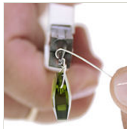
Step 14 Pull the wire around the round nose pliers until it is almost pointing directly down.
