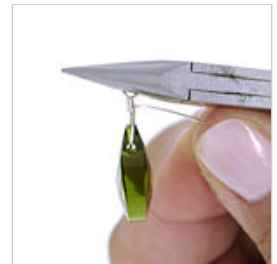
Step 18 Wrap the wire around the base wire. Continue wrapping the wire down to the first wrap.
