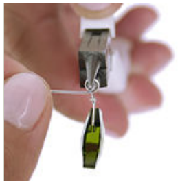
Step 16 Continue pulling the wire around the nose of the pliers until the loop is completely round.
