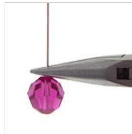
Step 2 Using the tips of your chain nose pliers, grab the wire directly above the beads.
